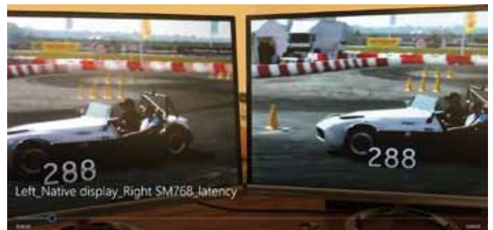
Fig. 3: testing side-by-side with a native display connection shows that the latency of the SM768 is invisible
