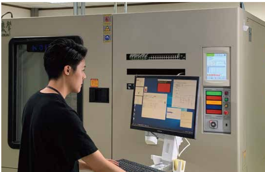
Figure 3: High and Low Temp. Stress Test with Chamber
