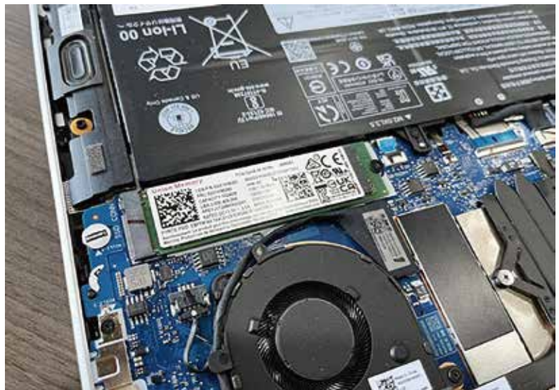
Figure 1: Solid State Disk (SSD) has become one of the core components of Notebooks.
